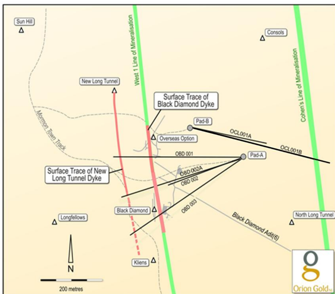
Figure 2: Schematic plan illustrating the position of mineralised trends in the Cohen's area, historic workings, the projected trend of the Black Diamond dyke and New Long Tunnel dyke and the location of drill holes.
